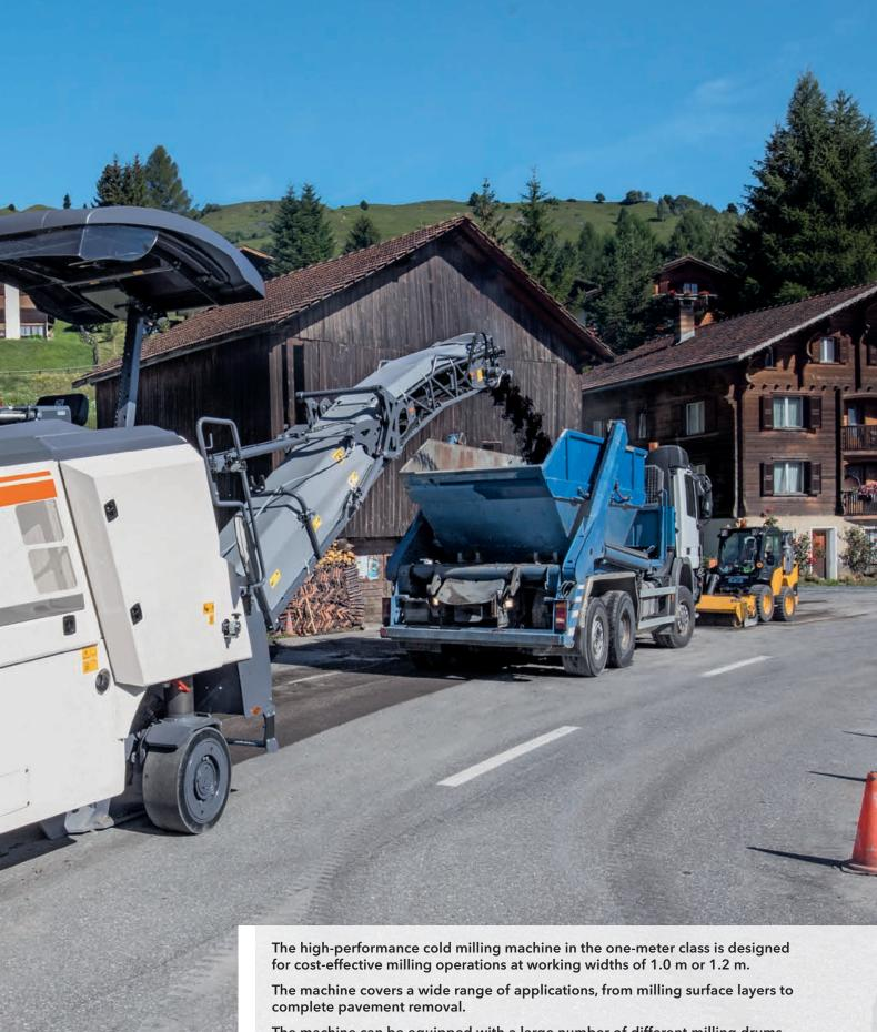
The machine can be equipped with a large number of different milling drums, increasing flexibility and machine utilization.
