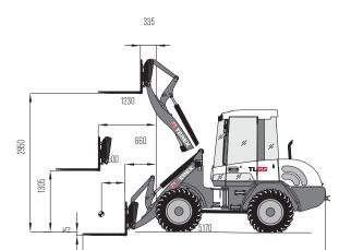
Operating load over total lift range: 1550 (1650\*) kg Operating load in transport position: 1900\* kg "With rear axle weights
