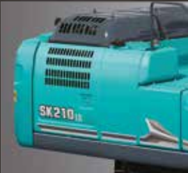
Panels and supports The right and left side panels and rear supports have been thicker to enhance body rigidity.
