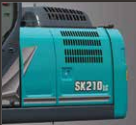
Panels and supports The right and left side panels and rear supports have been thicker to enhance body rigidity.
