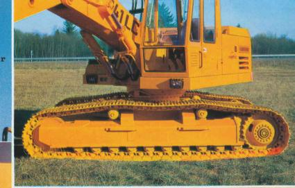
The running gear is entirely maintenance-free. Crawler tracks are hydraulically tensioned. The idler sprocked is spring loaded to cope with all forces exceeding the normal range of chain tensioner movement. The tracks are accurately guided by the sprocket wheels even under extreme loadings. You can choose between various track widths and grip patterns.
