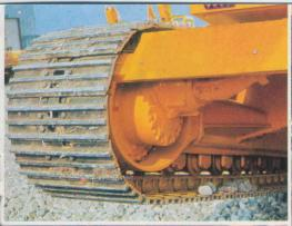
Each side of the excavator is driven by its own hydraulic power unit.
