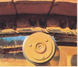
The crawler track support rollers are overhung from their bearings. The travel gear side members are thus effectively selfcleaning. The chains are less exposed to
