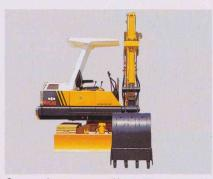
Convenient boom offset: The boom itself can be swung 90° to right side. As a result, PC40-5 is excellent in side digging in adjacent to the wall. In addition, it also can be swung 50° to left side. This means that PC40-5 can complete quick dig/load operation in extra tight quarters without swinging the upper structure.
