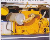
Komatsu-built 3D95S engine provides a tenacious power of 38 HP (28.7 kW) at 2600 RPM, and assures powerful excavation even at partial throttle, without the fear of stalling.
