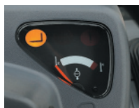
KOPS Plus Hydraulic Lock Indicator
