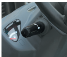
Finger-tip operation with the electric F/R lever
