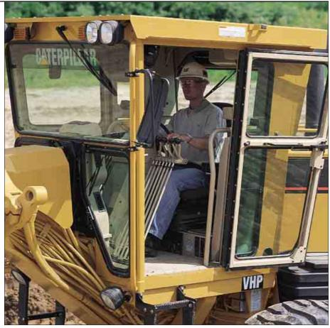
**Air Conditioner and Heater-Pressurizer.** The optional air conditioner arrangements help create a comfortable work environment. A cab heater-pressurizer is standard. The high-capacity systems dehumidify air and pressurize the cab, while circulating fresh air and sealing out dust. Multiple additional vents evenly distribute air throughout the cab for clear windows and operator comfort.
