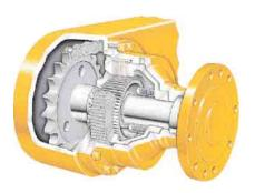
**Brakes.** Caterpillar multi-disc brakes offer a large surface area for dependable, extended-life braking. The air-actuated service brakes, located in each of the four wheel spindle housings, are sealed, adjustment free, and lubricated and cooled by tandem housing oil. The parking/ emergency brakes, located in the transmission on the output shaft, are spring actuated and air pressure released. When engaged, they neutralize the transmission and lock the wheels on any surface.
