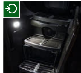
The entrance step lighting integrated on the side of the tank guarantees safe entering and exiting the cab.
