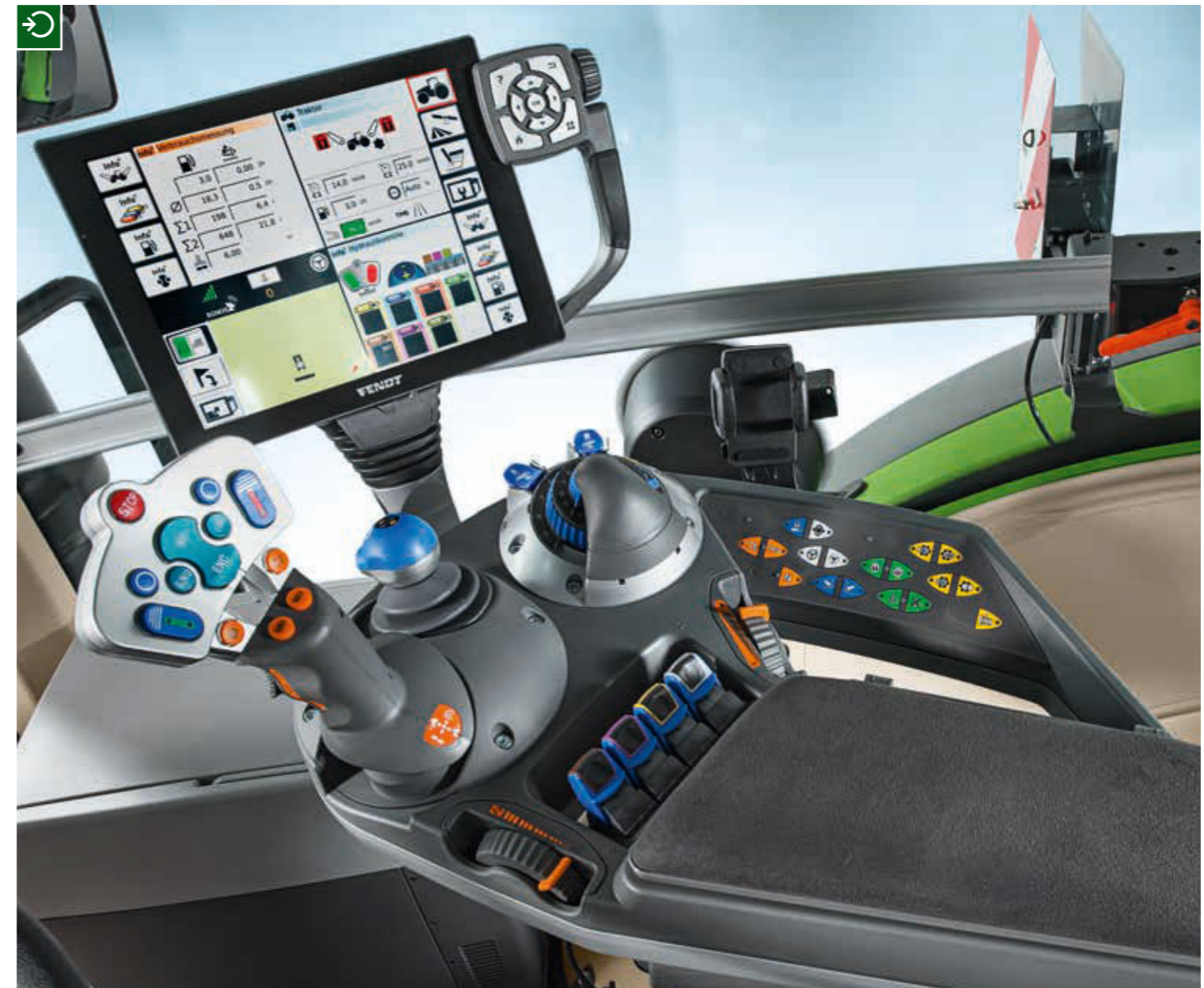
An ergonomic control centre comprising a 4-in-1 Varioterminal, multi-function joystick, crossgate lever, EPC power lift module, valve control and membrane keypad gives you easy access to everything you need.
