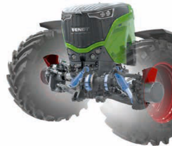
Front axle with self-levelling independent wheel suspension and single wheel brake
