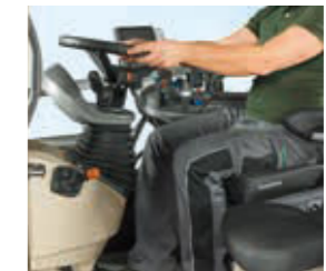
For enhanced operating comfort, the cockpit swings parallel with the steering wheel.
