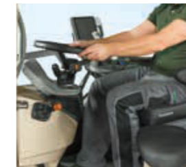
For enhanced operating comfort, the cockpit swings parallel with the steering wheel.
