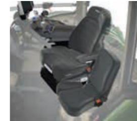
The new Dualmotion comfort seat Fendt Evolution with seat heater, climate control and Dualmotion swing-along backrest, is especially comfortable and ergonomic.
