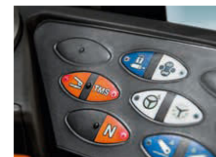
All functions are arranged simply and straightforward on the backlit membrane keypad according to the tried and tested Fendt operating logic.
