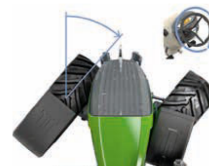
With VarioActive, you already go through the full steering angle with just one turn of the steering wheel.
