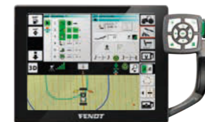
The Variotronic ® headland management saves all the procedures when performing a turning manoeuvre. Variotronic ® automatic triggers the sequences precisely at the right place.
