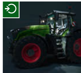
With the coming home function, the headlamps and the lights on the entry steps continue to shine after the engine has been turned off so that the way home as well as the steps are illuminated.
